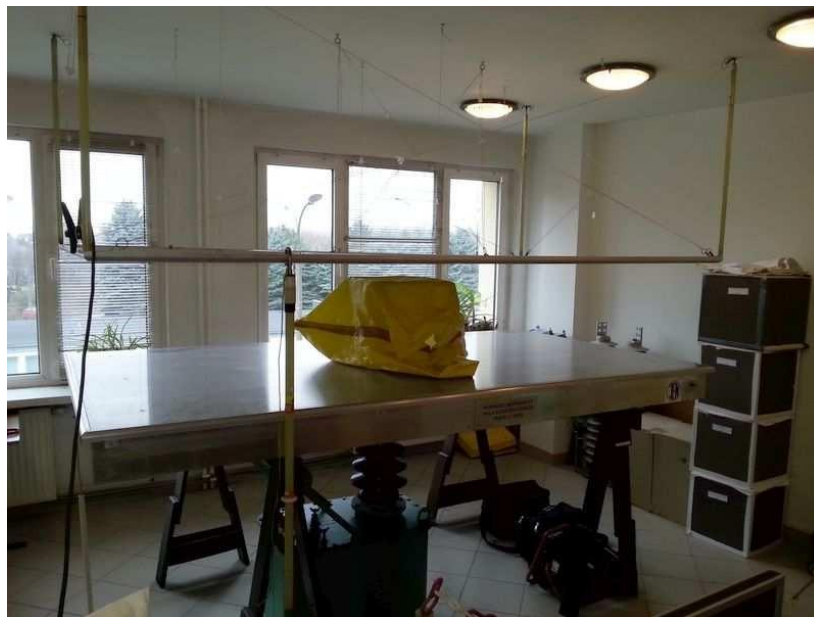
Image 1. Test bench for 50 Hz electric field meters
