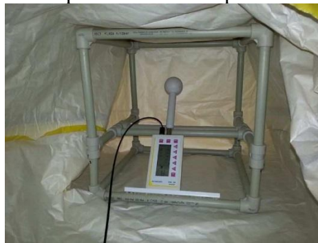
Image 2. View of the test setup with Maschek ESM-100 meter for testing of electrical field absorption during the test on the tester bench (Test Material 6, cage covered by construction-grade material, interior view)
