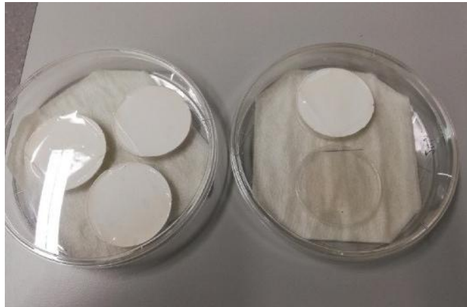
Fig-1. Paint samples and controls during incubation in Petri dishes.
